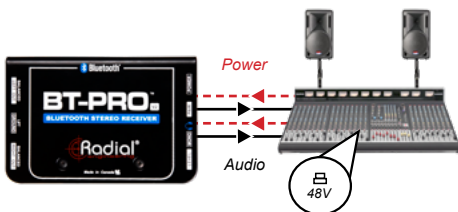
Powering the BT-Pro using 48V phantom power
