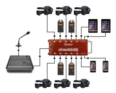
Several Exo-Pod units can also be linked together to expand to large numbers of outputs. Use a +4dB or hotter line-level output signal when feeding the first Exo-Pod for this purpose.
