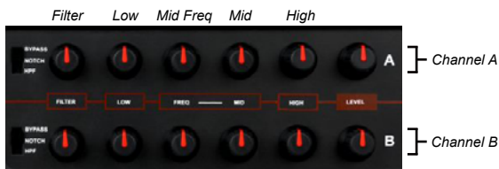
The dual EQ and Filter sections of the PZ-Pro
