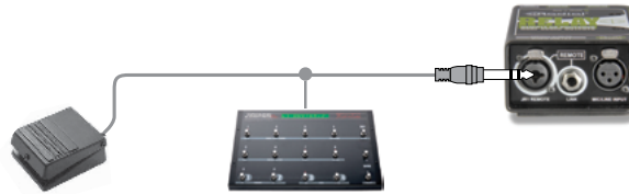
Simple footswitches and contact-closure devices like MIDI controllers use 1/4" cables to connect to the Relay Xo.
