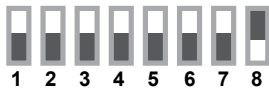
The EFX ON is in 'normal' mode when DIP switch #8 is in the UP position
