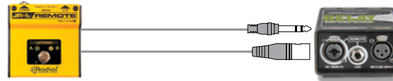
The JR1 uses either 1/4" or locking XLR cable to connect to the Relay Xo.
