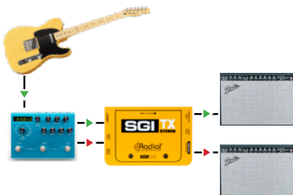
Using the SGI Stereo TX to feed local amplifiers when the RX isn't needed
