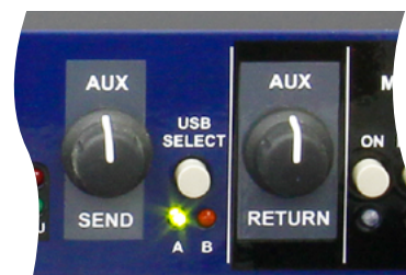
Front panel USB Select switch. Note that this switch will be inactive when an external footswitch is connected.
