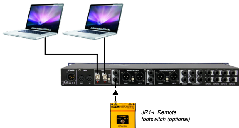
Using redundant laptops with the KL-8
