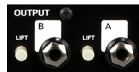
The amp outputs and lift switches
