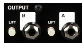
The amp outputs and lift switches
